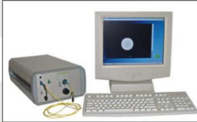
Core Eccentricity Measurement
